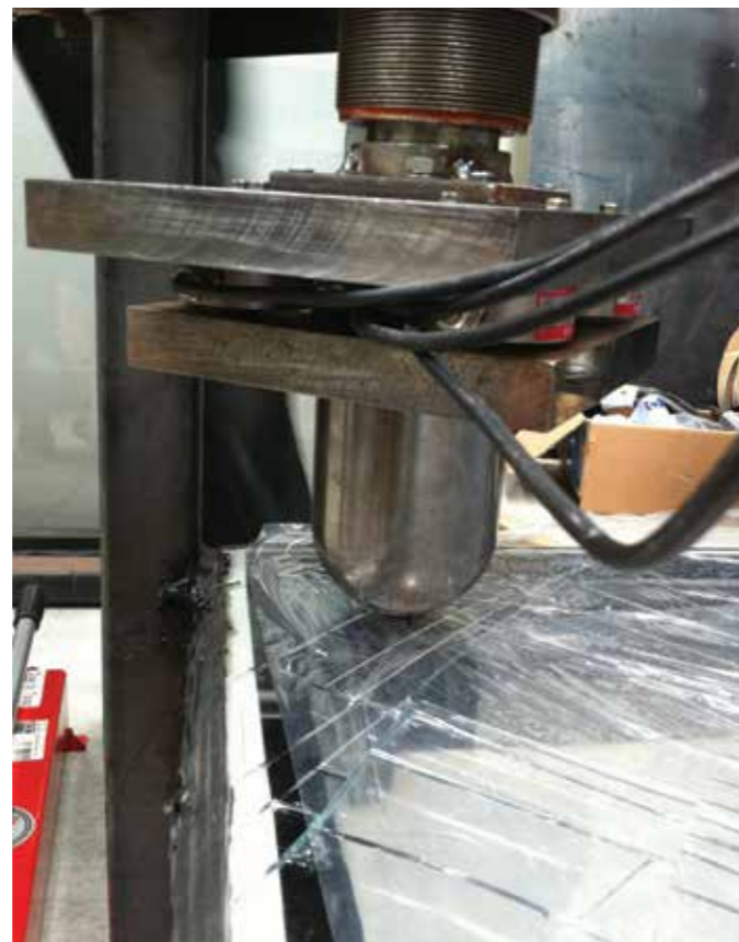
ArbourShield®-PG ARB28P under test where a 227kg solid steel weight is dropped from 2.8 metres...
